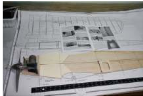
Layout the engine in the motor mount in order to get the correct spacing for the spinner and for the firewall. Remember to offset the firewall one degree right and down.
