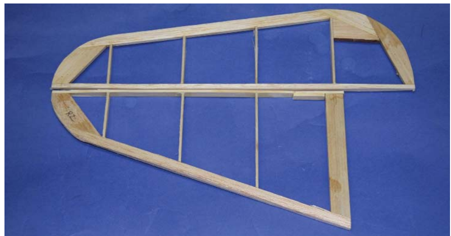
The elevator and rudder are built over the plan using 1/2 x 1/8-inch basswood strips (above, below). Balsa pre-cut end pieces form the rounded elevator and rudder ends. Joe used CyA medium and thin for both assemblies. Once dry he lined up the pieces and marked them for hinge location.
