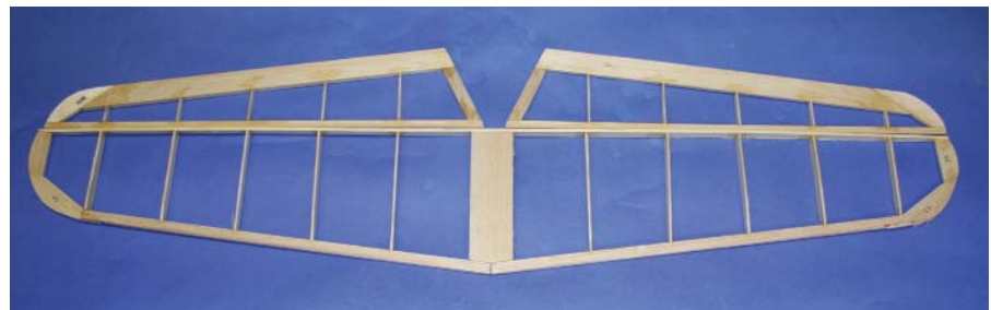
The elevator and rudder are built over the plan using 1/2 x 1/8-inch basswood strips (above, below). Balsa pre-cut end pieces form the rounded elevator and rudder ends. Joe used CyA medium and thin for both assemblies. Once dry he lined up the pieces and marked them for hinge location.
